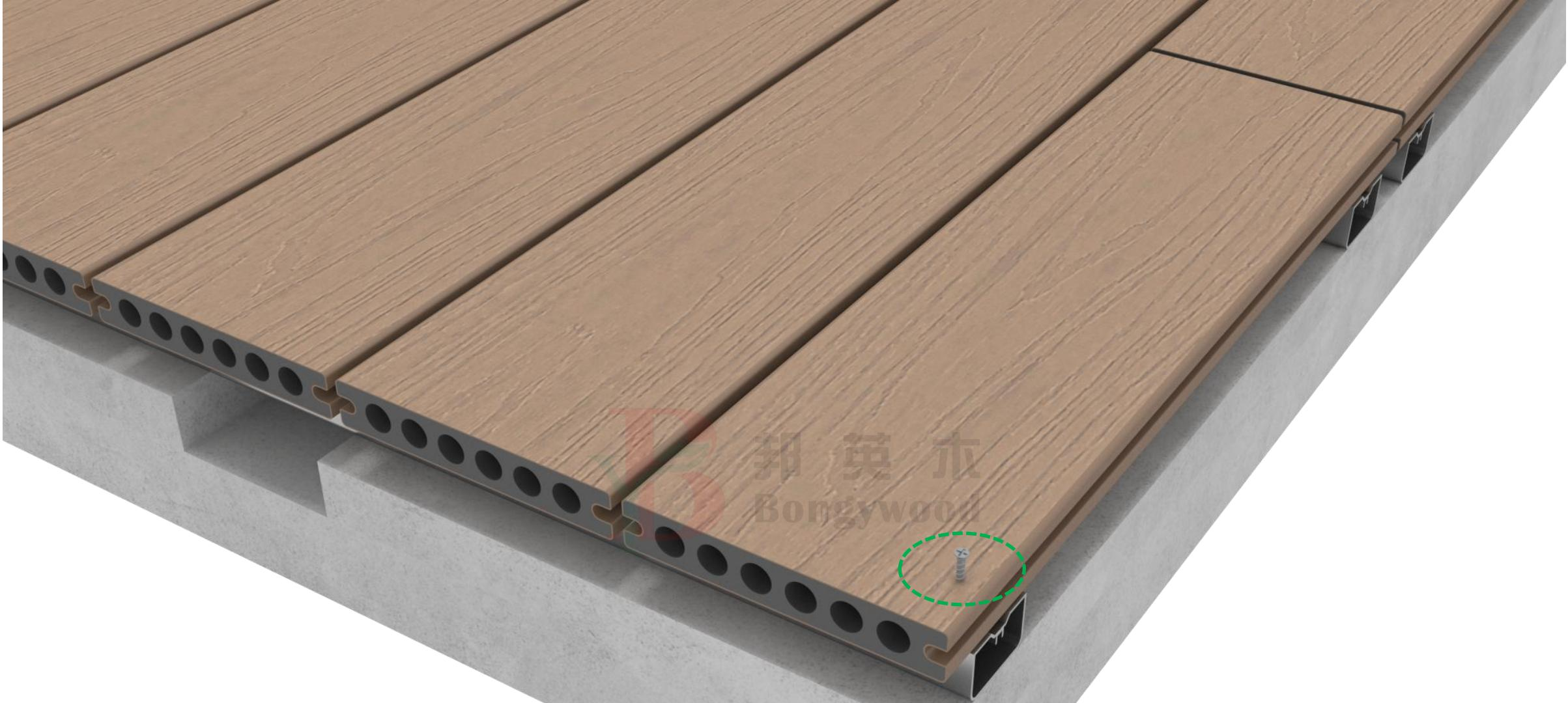
7. ①Fix the final decking in place using exposed screws driven through its face.
